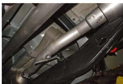
3. Install Headpipe # A onto use your factory clamp. Insert hanger into the rubber grommet. Do not tighten the clamp until install is complete.
