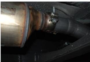
**5.** Install passenger side tailpipe #D to the muffler 1 1/2"-2". Use clamp #G to secure tailpipe to muffler. DO NOT TIGHTEN. Insert welded hangers into rubber grommet.
