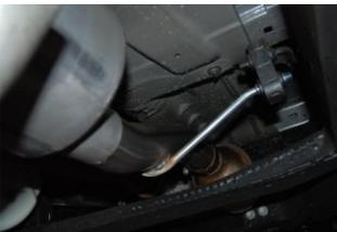
**4.** Install muffler #B onto head pipe 1 1/2"-2" with the louvers facing towards the converter. Use a jack stand to support the muffler. Use clamp #H to secure the muffler to the headpipe. DO NOT TIGHTEN. Muffler inlet is looking into the louvers.
