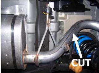
**2.** To remove the stock exhaust, remove it from clamp in front of the muffler. Do not discard you will re-use clamp. Disengage the welded hangers using WD-40 from the OEM rubber grommets. Do not damage or remove the rubber grommets as you will reuse them to mount your new system. Now, cut off tailpipe before and after rear axle for removal.
