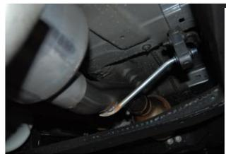
**3.** Clamp head pipe #A onto your existing stock front pipe re-using stock clamp. Use a jack stand to support the converter. Insert welded hanger into rubber grommet. DO NOT TIGHTEN.
