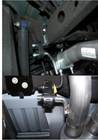
**7.** Install driver's side rear hanger #M onto side of frame as seen in picture. Secure bolt kit #O to frame. Use grommet #L and clamp hanger #N. This clamp also holds exit pipe to tailpipe.
