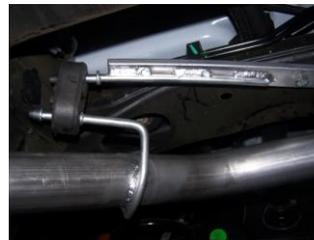
**9.** Install the exit pipes #E. Use clamp #H to secure exit pipes to tailpipes. DO NOT TIGHTEN.
