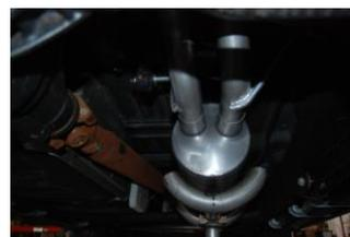
**5.** Install passenger side tailpipe #D to the muffler 1 1/2"-2". Use clamp #H to secure tailpipe to muffler. DO NOT TIGHTEN. Insert welded hangers into rubber grommets.
