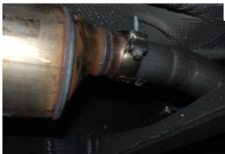
**4.** Install muffler #B onto head pipe #A 1 1/2"-2". Use a jack stand to support the muffler. Use clamp #G to secure the muffler to the headpipe. DO NOT TIGHTEN.
