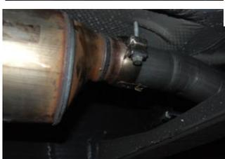
**5.** Install passenger side tailpipe #D to the muffler 1 1/2"-2". Use clamp #H to secure tailpipe to muffler. DO NOT TIGHTEN. Insert welded hangers into rubber grommets.
