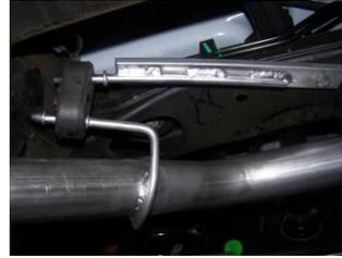
**6.** Install driver side rear hanger #I into hole located on cross member in front of spare tire.
