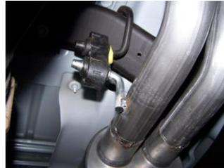
**6.** Install Driver side tailpipe #C into muffler outlet 1½"-2". Insert welded hanger into rubber grommet. Use clamp #F to attach tailpipe to muffler. DO NOT TIGHTEN.
