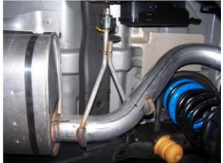
**2.** To remove the stock exhaust, remove it from the clamp in front of the muffler. Do not destroy you will re-use clamp. Disengage the welded hangers using WD-40 from the OEM rubber grommets. Do not damage or remove the rubber grommets as you will reuse them to mount your new system. Now, cut off tailpipe before and after rear axle for removal.
