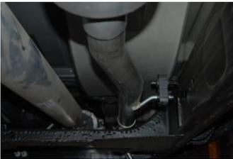
Next, install the headpipe #A into adapter pipe #F. Insert welded hanger into rubber grommet. Use clamp #E to secure together. **DO NOT TIGHTEN.**
