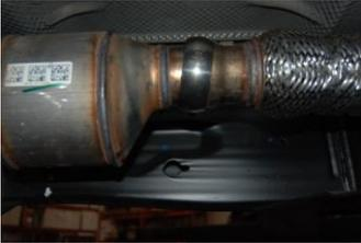
2. To remove stock exhaust, unclamp at the ball connection behind the Y-pipe. Make sure to leave all rubber grommets in the factory location. **You will re-use stock clamp.** For easier removal of exhaust, cut behind the muffler. Use WD-40 to remove hangers from 3. Bolt adapter pipe #F to the stock dome re-using the factory clamp. Do not tighten, just make snug.
