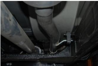
3. Bolt adapter #I to the stock flange re-using the factory into rubber grommet. Do not tighten.
