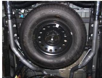
8. Install exit pipes #E onto tailpipes. Cut to your preferred length then use clamps to secure exit pipes to tailpipes. Install stainless steel tips. Clamp down. When you have everything in place, firmly tighten all bolts and clamps down securely. Use stainless steel cleaner and a Scotch Brite pad weekly to prevent tip from discoloration. Inspect all fasteners after 25-50 miles of operation and re-tighten as necessary.
