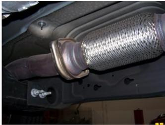
2. Remove the stock exhaust by unbolting it at the flange located in front of the muffler. Disengage the welded hangers from the OEM rubber grommets. Use WD-40 to aid in this process. Do not damage stock nuts and bolts or remove the rubber grommets as you will re-use them to mount your new system. Now, cut off tailpipe and remove system.
