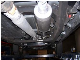
4. Install muffler #B onto headpipe 1½"-2" with the louvers facing towards the converter. Use a jack stand to support the muffler. Use clamp #G to secure the muffler to the headpipe. Do not tighten. Muffler inlet is looking into the louvers.
