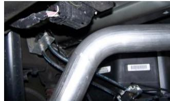
7. Slide driver side tailpipe #D into muffler 1½"-2" and secure with clamp #F. Do not tighten. Insert welded hangers into rubber grommets.
