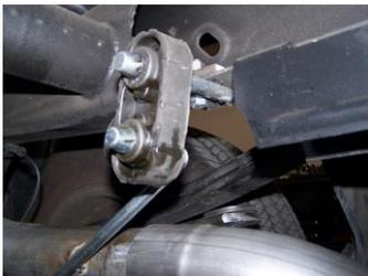
5. Next, remove your spare tire. Then install passenger side tailpipe hanger #I. You will see a 1½" hole in the frame. Attach hanger to this hole and re-install factory grommet on hanger.
