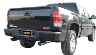
10. If you haven't done so already ... Install stainless steel tips. Clamp down. When you have everything in place, firmly tighten all bolts and clamps down securely. Use stainless steel or aluminum cleaner to polish tips. Inspect all fasteners after 25-50 miles of operation and re-tighten as necessary.
