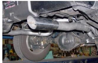
9. Slide each exit pipe #E onto each tailpipe 1.5-2" and secure with clamp #H. Do not tighten. Rotate exit pipes to best suit your vehicle. It is best to adjust these pipes with the tips already on the pipes. That way you can make sure there is proper clearance.
