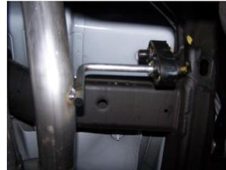
**5.** Install Passenger side tailpipe #D into muffler outlet 1 1/2"-2". Insert welded hangers into rubber grommets. Use clamp #F to attach to tailpipe to muffler. DO NOT TIGHTEN.
