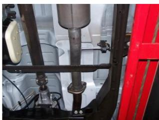
**4.** Install muffler #B onto head pipe #A 1 1/2"-2". Muffler outlets will be positioned at the top. Use a jack stand to support the muffler. Use clamp #E to secure the muffler to the headpipe. DO NOT TIGHTEN.
