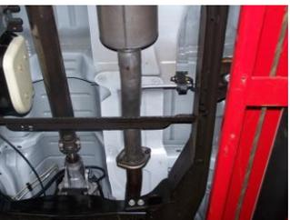
**4.** Install muffler #B onto head pipe #A 1½"-2". Use a jack stand to support the muffler. Muffler outlets will be positioned at the top. Use clamp #F to secure the muffler to the headpipe. DO NOT TIGHTEN.
