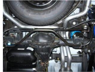
**7.** Install driver side tailpipe #C into the muffler 1½-2". Use clamp #G to secure tailpipe to muffler. DO NOT TIGHTEN. Insert welded hangers into rubber grommets.
