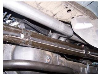
**8.** Install the exit pipes #E. Use clamp #G to secure exit pipes to tailpipes. DO NOT TIGHTEN. Rotate pipes to adjust for desired look. Re-install spare tire.
