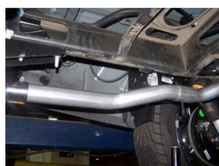
**5.** Remove spare tire to install tailpipes. Now install passenger side tailpipe #D into the muffler 1½-2". Use clamp #G to secure tailpipe to muffler. DO NOT TIGHTEN. Insert welded hangers into rubber grommets.
