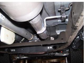
Bolt head pipe #A onto your existing stock front pipe re-using stock bolts. Insert welded hanger into rubber grommet. DO NOT TIGHTEN.
