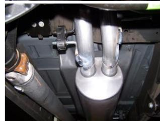
**9.** Install stainless steel tips #J. Clamp down. When you have everything in place, firmly tighten all bolts and clamps down securely. Use stainless steel cleaner and a Scotch Brite pad weekly to prevent tip from discoloration. Inspect all fasteners after 25-50 miles of operation and re-tighten as necessary.
