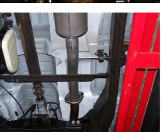
**4.** Install muffler #B onto head pipe #A 1½"-2". Use a jack stand to support the muffler. Muffler outlets will be positioned at the top. Use clamp #F to secure the muffler to the headpipe. DO NOT TIGHTEN.
