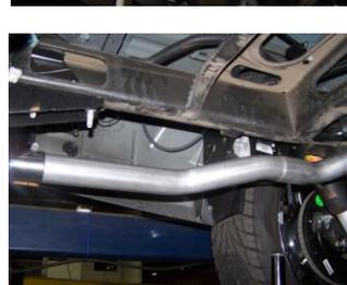
**5.** Remove spare tire to install tailpipes. Now install passenger side tailpipe #D into the muffler 1½-2". Use clamp #G to secure tailpipe to muffler. DO NOT TIGHTEN. Insert welded hangers into rubber grommets.
