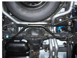
**7.** Install driver side tailpipe #C into the muffler 1 1/2"-2". Use clamp #G to secure tailpipe to muffler. DO NOT TIGHTEN. Insert welded hangers into rubber grommets.
