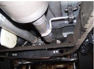
**4.** Install muffler #B onto head pipe 1 1/2"-2" with the louvers facing towards the converter. Use a jack stand to support the muffler. Muffler outlets will be positioned at the top. Use clamp #F to secure the muffler to the headpipe. DO NOT TIGHTEN.
