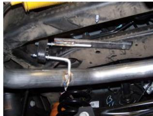
**6.** Install driver side rear hanger #H into hole located on cross member behind spare tire location (see photo). Use bolt kit #I to secure and attach Rubber grommet #L. DO NOT TIGHTEN.
