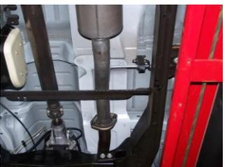
**5.** Remove spare tire to install tailpipes. Now install passenger side tailpipe #D into the muffler 1 1/2"-2". Use clamp #G to secure tailpipe to muffler. DO NOT TIGHTEN. Insert welded hangers into rubber grommets.
