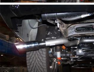
**9.** Install stainless steel tips #J. Clamp down. When you have everything in place, firmly tighten all bolts and clamps down securely. Use stainless steel cleaner and a Scotch Brite pad weekly to prevent tip from discoloration. Inspect all fasteners after 25-50 miles of operation and re-tighten as necessary.
