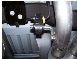
**8.** Install driver side tailpipe #C to the muffler 1 1/2"-2". Use clamp #H to secure tailpipe to muffler. DO NOT TIGHTEN. Insert welded hangers into rubber grommets.
