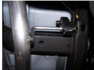
**5.** Install passenger side tailpipe #D to the muffler 1 1/2"-2". Use clamp #H to secure tailpipe to muffler. DO NOT TIGHTEN. Insert welded hangers into rubber grommets.
