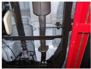
**4.** Install muffler #B onto head pipe #A 1 1/2"-2". Use a jack stand to support the muffler. Use clamp #G to secure the muffler to the headpipe. DO NOT TIGHTEN.
