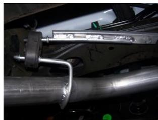
**6.** Install driver side rear hanger #I into hole located on cross member in front of spare tire.
