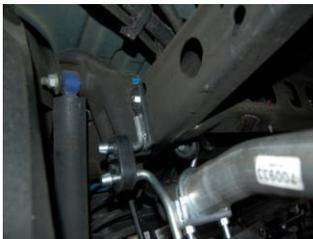
**7.** Install driver's side rear hanger #M onto side of frame as seen in picture. Secure bolt kit #O to frame. Use grommet #L and clamp hanger #N. This clamp also holds exit pipe to tailpipe.
