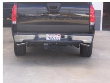
INSTALL STAINLESS TIPS. CLAMP DOWN. WHEN YOU HAVE EVERYTHING IN PLACE, FIRMLY TIGHTEN ALL BOLTS AND CLAMPS DOWN SECURELY. TO CLEAN TIPS, USE A STAINLESS STEEL CLEANER AND A SCOTCH BRITE PAD.
