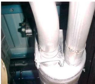
Next, install rear muffler hanger #H onto driverside muffler outlet insert hanger into rubber grommet. Do not tighten.
