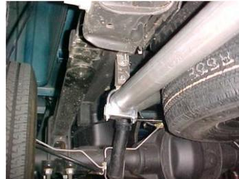
Install exit pipes #F Use clamps # I to secure exit pipes to tailpipes. These clamps also attach to the metal hangers. You will need to rotate in order to adjust for clamping.
