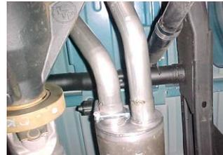
Install tailpipe hangers #J onto end of tailpipes using clamp #I. There will be about a 2" hole above the end of both tailpipes on the frame to bolt the hangers. Do not tighten.
