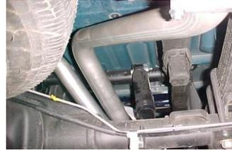
Install passenger side overaxle tailpipe #D into muffler 1 1/2" to 2". Long end of pipe goes into muffler Secure with clamp #I. Do not tighten.
