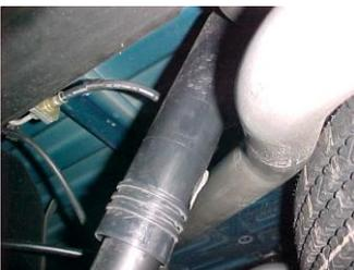
Install driverside overaxle tailpipe #E into muffler 1 1/2" to 2". Long end of pipe goes into the muffler. Support end of tailpipe with stand, and attach with hanger # H.
