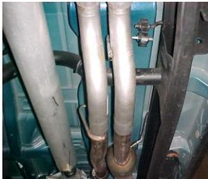
Install driverside headpipe #B. Then install headpipe #A. And then Insert welded hanger into rubber grommet. Secure both pipes with clamp #G. Do not tighten.
