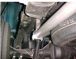
Install tailpipe hangers #J onto end of tailpipes using clamp #I. There will be about a 2" hole above the end of both tailpipes on the frame to bolt the hangers. Do not tighten.
