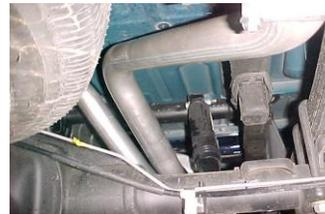
Install passenger side overaxle tailpipe #D into muffler 1 1/2" to 2". Long end of pipe goes into muffler. Secure with clamp #I. Do not tighten.
