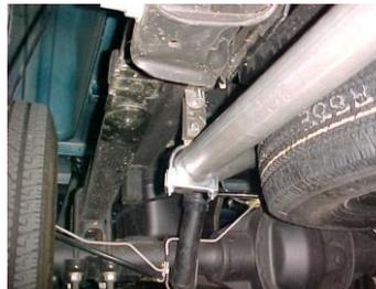
Install exit pipes #F Use clamps # I to attach to tailpipes. These clamps also attach to the metal hangers # J. You will need to rotate in order to adjust for clamping.
