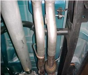
Install driverside headpipe #B. Then install headpipe #A and then Insert welded hanger into rubber grommet Secure both pipes with clamp #H. Do not tighten.
