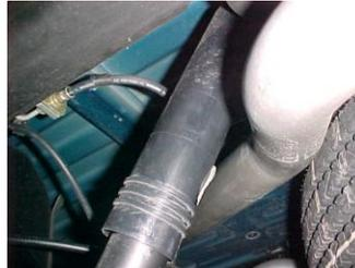
Install driverside overaxle tailpipe #E into muffler 1 1/2" to 2". Use clamp #I to secure pipe to muffler. Do not tighten. Next, insert welded hanger into rubber grommet. Rotate pipe until it connects with rear hanger. Attach clamp #I to tail pipe.
