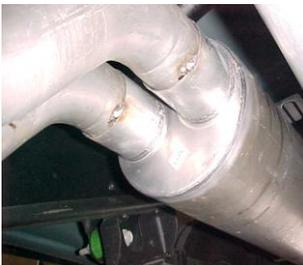
Install muffler # C onto head pipes 1-1/2" to 2" with the louvers facing towards the converter. Use a jack stand to support the muffler. Use clamps #G to secure the muffler to the head pipes. Do not tighten. Outlets will be on the bottom.
