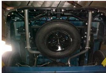
Now go back and tighten all clamps, nuts and bolts. Start from the front and work back.
