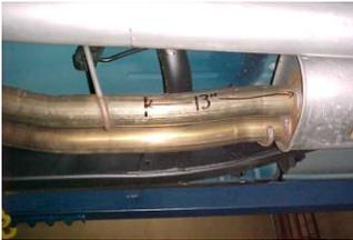
Lay out the exhaust on the floor so it looks like the drawing and compare parts with manual. **To remove the stock exhaust cut 13" just in front of the muffler.**
