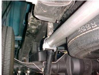
Install exit pipes #F Use clamps # H to secure exit pipes to tailpipes. These clamps also attach to the metal hangers. You will need to rotate in order to adjust for clamping.
