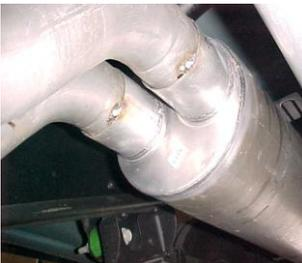
Install muffler # C onto head pipes 1-1/2" to 2" with the louvers facing towards the converter. The outlets of the muffler will be on top. Use a jack stand to support the muffler. Use clamps #G to secure the muffler to the head pipes. Do not tighten
