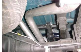
Install passenger side overaxle tailpipe #D into muffler 1 1/2" to 2". Secure with clamp #H. Do not tighten.
