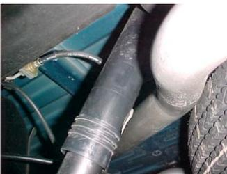
Install driverside overaxle tailpipe #E into muffler 1 1/2" to 2". Support end of tailpipe with stand, and attach with hanger # H.
