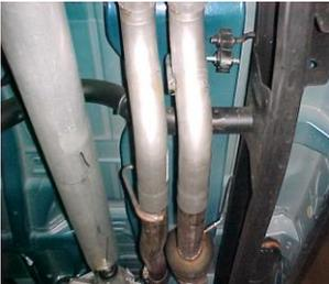
Install driverside headpipe #B onto factory pipe. Then install headpipe #A onto factory pipe. Insert welded hanger into rubber grommet. Secure both pipes with clamp #G. Do not tighten.
