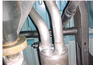
Install tailpipe hangers #I onto end of tailpipes using clamp #H. There will be about a 2" hole above the end of both tailpipes on the frame to bolt the hangers. Do not tighten.
