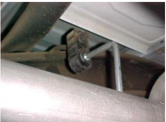
Install head pipe # A onto you're existing stock flange use your factory hardware. Use a jack stand to support the converter. Insert welded hanger into rubber grommet. Do not tighten.
