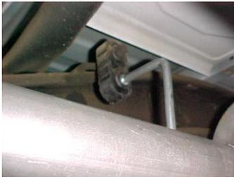
Install head pipe # A onto your existing stock flange use your factory hardware. Use a jack stand to support the converter. Insert welded hanger into rubber grommet. Do not tighten.
