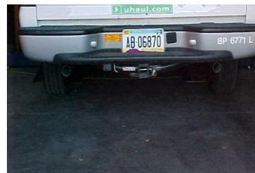
Install exit pipes # E Use clamps # H to secure exit pipes to tailpipes. These clamps also attach to the metal hangers # I. You will need to rotate in order to adjust for clamping. Now go back and tighten all clamps, nuts and bolts. Start from the front and work back. Install Stainless tips
