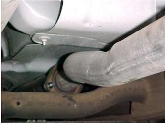
Lay out the exhaust on the floor so it looks like the drawing and compare parts with manual. To remove the stock exhaust remove it from the 2-bolt flange located in front of the muffler. **You will re-use your stock hardware.** Leave all rubber grommets in place. Use WD-40 to aid in removal of exhaust and hangers. Use hacksaw to cut tailpipe off.
