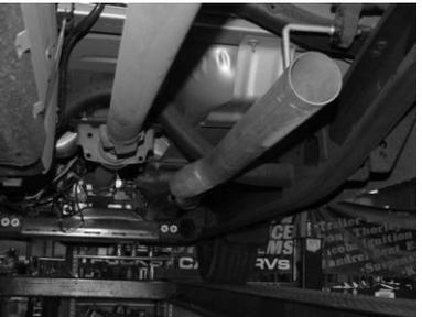
INSTALL PASSENGER SIDE TAILPIPE #C INTO MUFFLER AT LEAST 1 1/2" TO 2". USE CLAMP #G TO SECURE PIPE TO MUFFLER. DO NOT TIGHTEN. THE TAILPIPES WILL BOTH LEAN TOWARDS THE DRIVER SIDE. LOOKING FROM THE REAR OF THE VEHICLE - THIS TAILPIPE IS AT APPX. 11 O'CLOCK.
