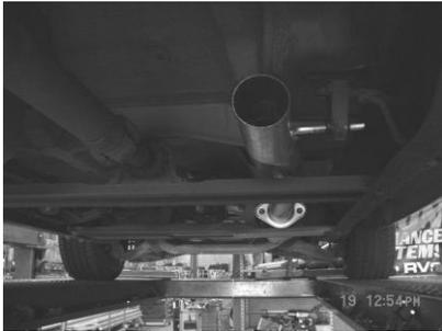
BOLT THE HEADPIPE #A ONTO FACTORY FLANGE USING GASKET #K AND RE-USING THE FACTORY NUTS AND BOLTS. SLIDE THE WELDED HANGER INTO THE RUBBER GROMMET. DO NOT TIGHTEN. INSTALL MUFFLER ON TO THE HEADPIPE 1- 1/2" TO 2" WITH INLET TOWARDS CONVERTER USING CLAMP #F TO SECURE MUFFLER TO HEADPIPE. USE A JACKSTAND TO SUPPORT THE MUFFLER. DO NOT TIGHTEN.
