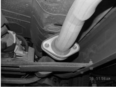
UNBOLT THE 2-BOLT FLANGE LOCATED BEHIND THE CONVERTER, **SAVE STOCK NUTS AND BOLTS FOR YOU WILL REUSE THEM.** NOW CUT OFF YOUR STOCK TAILPIPE JUST BEHIND THE MUFFLER AND REMOVE. USE WD-40 TO AID IN REMOVAL OF THE EXHAUST AND HANGERS. LEAVE ALL RUBBER GROMMETS ON THE HANGER.
