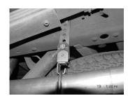
REMOVE STOCK REAR HANGER FROM FRAME ON PASSENGER SIDE. INSTALL 10" METAL HANGER #H. USE THE FIFTH HOLE FROM THE BOTTOM. INSTALL IT IN THE FACTORY HOLE WHERE THE STOCK HANGER WAS IN. IT IS LOCATED APPROX. 20" FROM REAR OF FRAME 3/8" HOLE.
