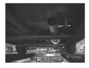
BOLT THE HEADPIPE #A ONTO FACTORY FLANGE USING GASKET #L AND RE-USING THE FACTORY NUTS AND BOLTS. SLIDE THE WELDED HANGER INTO THE RUBBER GROMMET. DO NOT TIGHTEN. INSTALL MUFFLER ON TO THE HEADPIPE 1- 1/2" TO 2" WITH INLET TOWARDS CONVERTER USING CLAMP #F TO SECURE MUFFLER TO HEADPIPE. USE A JACKSTAND TO SUPPORT THE MUFFLER. DO NOT TIGHTEN.
