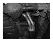
INSTALL PASSENGER SIDE TAILPIPE #C INTO MUFFLER 1-1/2" TO 2" USING CLAMP #G. ATTACH CLAMP #G TO TAILPIPE AND SECURE WITH HANGER #H.THIS WILL HOLD UP THE PIPE. DO NOT TIGHTEN.
