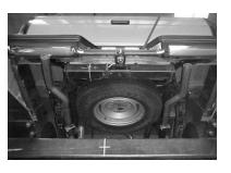
Install exit pipes # E onto the over axle pipes and attach with clamp #G. You may need to cut the exit pipes to your preference. Rotate all pipes until you have a minimum of a 1" clearance on all pipes. Use zip ties to reroute vent lines and brake lines. Tighten all clamps, flanges, bolts firmly. Install Stainless steel tips.
