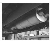
Install muffler #B onto the head pipe no more then 1 1/2" to 2". Use a jack stand to support the muffler. Make sure muffler is sitting level with the vehicle and that the muffler outlets are positioned level. Level outlets are at 12'oclock position. Attach headpipe with clamp
