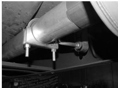
3.) SLIP MUFFLER #B ONTO THE HEADPIPE 1-1/2" TO 2" WITH INLET TOWARDS THE CONVERTER. USE A JACK STAND TO SUPPORT THE MUFFLER. USE CLAMP #H TO SECURE MUFFLER TO HEADPIPE. DO NOT TIGHTEN. ATTACH HANGER #F TO HEADPIPE.
