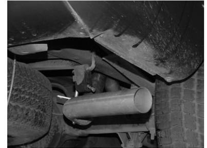
6.) INSTALL DRIVERSIDE OVERAXLE TAILPIPE #D INTO MUFFLER 1-1/2" TO 2-1/2" AND SECURE PIPE TO MUFFLER USING CLAMP #I. NOW, BOLT BOTH PIPES TO THE TOGETHER USING BOLT KIT #J. DRIVERSIDE TAB MOUNT GOES ON THE BOTTOM. SPARE TIRE MAY NEED TO BE LOOSENED UP AND PUSHED OVER TO THE DRIVERSIDE.
