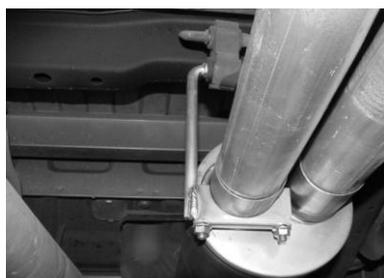
5.) INSTALL PASSENGER SIDE OVERAXLE TAILPIPE #C INTO MUFFLER 1-1/2" TO 2-1/2". SLIDE WELDED HANGER INTO RUBBER GROMMET. USE CLAMP #I TO SECURE PIPE TO MUFFLER. DO NOT TIGHTEN.
