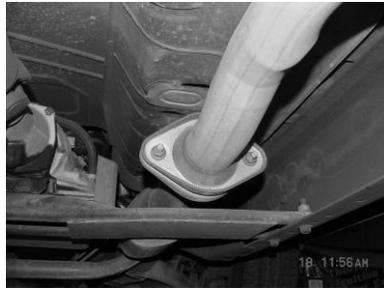
2.) BOLT HEADPIPE #A ONTO THE FACTORY FLANGE USING THE GASKET #K, NUTS & BOLTS. INSERT WELDED HANGER INTO RUBBER GROMMET. DO NOT TIGHTEN.
