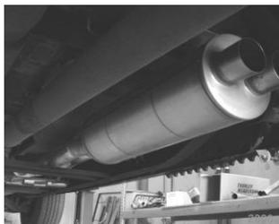
Install muffler #B onto the head pipe no more than 1-1/2" to 2". Use a jack stand to support the muffler. Make sure muffler is sitting level with the vehicle and that the muffler outlets are positioned level. Level outlets are at 12'oclock position. Attach to headpipe with clamp #f.
