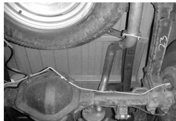
Slip the over axle tailpipes #C, #D into the outlets of the muffler no more than 1- 1/2" to 2" and attach clamp # G to passenger side and clamp hanger # I to driver side tailpipe. The driver side tailpipe will be routed over the differential between the frame and the shock. It will require some rotating of the pipe and possibly an extra person to help align the pipes when tightening the clamps. Attach hanger #H to tailpipes and attach with clamp #G.
