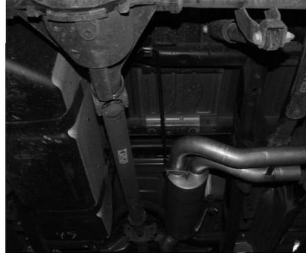
ROTATE THE MUFFLER ASSEMBLY UNTIL THE OUTLETS ARE LEVEL.
