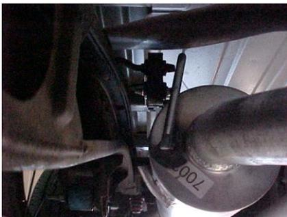
INSERT MUFFLER ASSEMBLY #A ONTO HEADPIPE AT LEAST 1-1/2" TO 2", USE A JACKSTAND TO SUPPORT MUFFLER ASSEMBLY. USE CLAMP #C TO SECURE MUFFLER ASSEMBLY TO THE HEADPIPE, DO NOT TIGHTEN. INSERT WELDED HANGER INTO RUBBER GROMMET.
