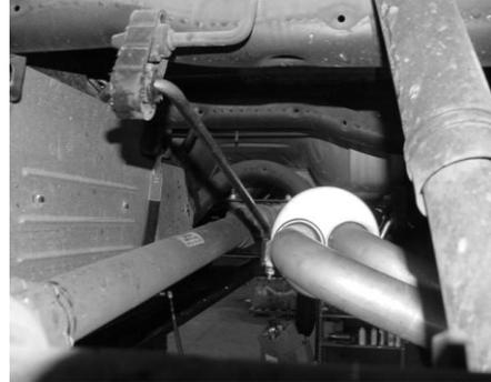
INSTALL HANGER #F INTO RUBBER GROMMET LOCATED JUST ABOVE TAILPIPE ASSEMBLY, SLIDE CLAMP THAT IS WELDED TO THE HANGER OVER DRIVERSIDE TAILPIPE, DO NOT TIGHTEN.
