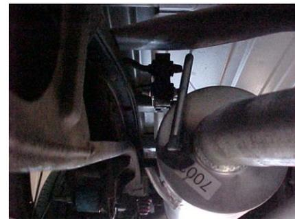
INSERT MUFFLER ASSEMBLY #B ONTO HEADPIPE AT LEAST 1-1/2" TO 2", USE A JACKSTAND TO SUPPORT MUFFLER ASSEMBLY. USE CLAMP #E TO SECURE MUFFLER ASSEMBLY TO THE HEADPIPE, DO NOT TIGHTEN. INSERT WELDED HANGER INTO RUBBER GROMMET.
