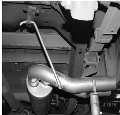
SLIDE MUFFLER ASSEMBLY ONTO HEADPIPE 1 1/2" TO 2". INSERT WELDED HANGER INTO RUBBER GROMMET ON DRIVERSIDE USE CLAMP #C TO SECURE MUFFLER TO HEADPIPE. DO NOT TIGHTEN.
