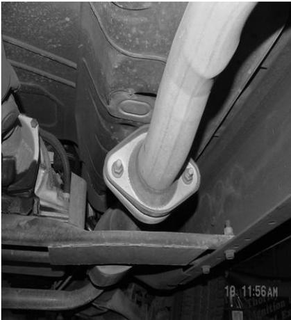
TO REMOVE EXHAUST- UNBOLT THE 2 BOLT FLANGE LOCATED BEHIND THE CATALYTIC CONVERTER. **SAVE STOCK NUTS AND BOLTS FOR YOU WILL REUSE THEM.** NOW CUT OFF YOUR STOCK TAILPIPE JUST BEHIND THE MUFFLER AND REMOVE. LEAVE ALL RUBBER GROMMETS ON THE HANGER. USE WD-40 TO AID IN THE REMOVAL OF THE EXHAUST AND HANGERS.
