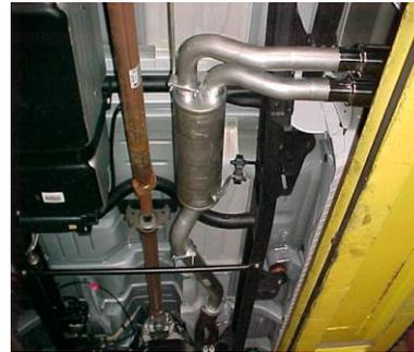
INSTALL MUFFLER ASSEMBLY #B ONTO HEADPIPE #A. SLIDE WELDED HANGERS INTO RUBBER GROMMETS. USE CLAMP #C TO SECURE MUFFLER ASSEMBLY TO HEADPIPE. **DO NOT TIGHTEN.**
