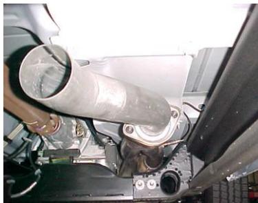
INSTALL HEADPIPE #A ONTO YOUR EXISTING STOCK 2-BOLT FLANGE. USE YOUR STOCK HARDWARE TO SECURE. DO NOT TIGHTEN. USE A JACK STAND TO SUPPORT THE CONVERTER.
