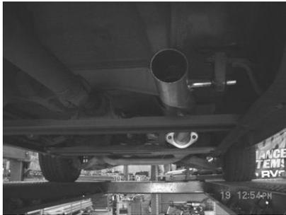
BOLT THE HEADPIPE #A ONTO FACTORY FLANGE RE-USING THE FACTORY NUTS AND BOLTS. SLIDE THE WELDED HANGER INTO THE RUBBER GROMMET. ATTACH HANGER #F TO HEADPIPE. DO NOT TIGHTEN.
