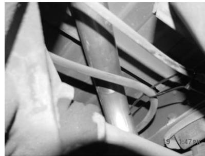
INSTALL PASSENGER SIDE TAILPIPE #C INTO MUFFLER 1-1/2" TO 2" USING CLAMP #I THEN ATTACH WITH CLAMP #H AND ATTACH TO MUFFLER. ATTACH HANGERS #I TO BOTH TAILPIPES. ATTACH WITH CLAMP #H. DO NOT TIGHTEN.
