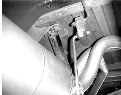
INSTALL REAR MUFFLER HANGER #J ONTO DRIVERS SIDE MUFFLER OUTLET. INSERT THE WELDED HANGER INTO RUBBER GROMMET. DO NOT TIGHTEN. INSTALL DRIVERSIDE TAILPIPE #D INTO MUFFLER 1-1/2" TO 2". THIS PIPE GOES BETWEEN THE SHOCK & FRAME. SLIDE CLAMP #H OVER PIPE AND CONNECT IT TO THE HANGER#I. THIS WILL HOLD UP THE TAILPIPE.
