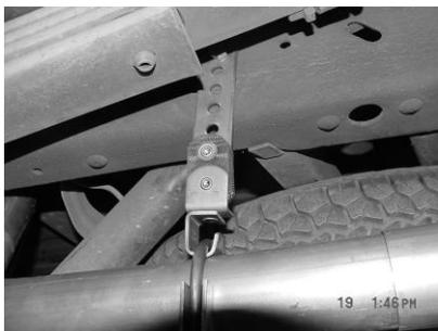
REMOVE STOCK REAR HANGER FROM FRAME ON PASSENGER SIDE. INSTALL 10" METAL HANGER #I. USE THE FIFTH HOLE FROM THE BOTTOM. INSTALL IT IN THE TOP FACTORY HOLE WHERE THE STOCK HANGER WAS IN. IT IS LOCATED APPROX. 20" FROM REAR OF FRAME 3/8" HOLE. REPEAT FOR THE DRIVERSIDE.
