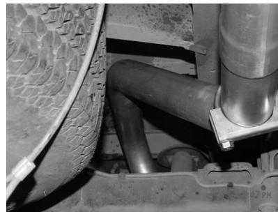
INSTALL EXIT PIPES #E ONTO TAILPIPES. ROLL EXIT PIPES UNTIL YOU HAVE THE CORRECT ANGLE. USE CLAMP #H TO SECURE THESE TO THE TAILPIPE. DO NOT TIGHTEN. CUT EXIT PIPE TO PROPER LENGTH.
