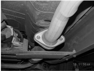
UNBOLT THE 2-BOLT FLANGE LOCATED BEHIND THE CONVERTER, **SAVE STOCK NUTS AND BOLTS FOR YOU WILL REUSE THEM.** NOW CUT OFF YOUR STOCK TAILPIPE JUST BEHIND THE MUFFLER AND REMOVE. USE WD-40 TO AID IN REMOVAL OF THE EXHAUST AND HANGERS. LEAVE ALL RUBBER GROMMETS ON THE HANGER. YOU NEED TO SUPPORT THE CONVERTER SO THE SYSTEM WILL NOT SIT ON THE CROSSMEMBER.
