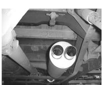
UNBOLT THE 2-BOLT FLANGE LOCATED BEHIND THE CONVERTER, SAVE STOCK NUTS AND BOLTS FOR YOU WILL REUSE THEM. NOW CUT OFF YOUR STOCK TAILPIPE JUST BEHIND THE MUFFLER AND REMOVE. USE WD-40 TO AID IN REMOVAL OF THE EXHAUST AND HANGERS. LEAVE ALL RUBBER GROMMETS ON
