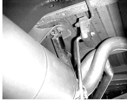
INSTALL REAR MUFFLER HANGER #J ONTO DRIVERS SIDE MUFFLER OUTLET. INSERT THE WELDED HANGER INTO RUBBER GROMMET. DO NOT TIGHTEN. INSTALL DRIVERSIDE TAILPIPE #D INTO MUFFLER 1-1/2" TO 2". PIPE GOES BETWEEN THE SHOCK & FRAME. SLIDE CLAMP #H OVER PIPE AND CONNECT IT TO THE HANGER#J. THIS WILL HOLD UP THE TAILPIPE.
