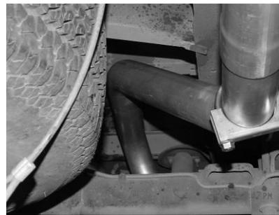
INSTALL EXIT PIPES #E C INTO TAILPIPES. ROLL EXIT PIPES UNTIL YOU HAVE THE CORRECT ANGLE. USE CLAMP #H TO SECURE THESE TO THE TAILPIPE. DO NOT TIGHTEN. CUT EXIT PIPE TO PROPER LENGTH.
