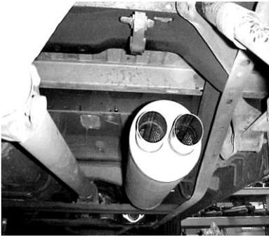
INSTALL MUFFLER #B ON TO THE HEADPIPE 1- 1/2" TO 2" WITH INLET TOWARDS CONVERTER USING CLAMP #G TO SECURE MUFFLER TO HEADPIPE. USE A JACKSTAND TO SUPPORT THE MUFFLER. DO NOT TIGHTEN.
