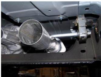
3. Install headpipe #A onto your existing stock flange and attach using stock hardware. Do not tighten. Insert welded hanger into rubber grommet.
