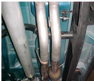
Install driverside headpipe #B. Then install headpipe #A and insert welded hanger into rubber grommet. Secure both pipes with clamp #G. Do not tighten.
