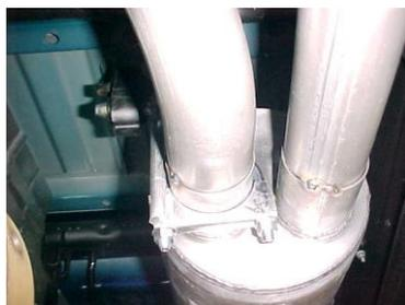
Next, install rear muffler hanger #H onto drivers side muffler outlet and insert hanger into rubber grommet. Do not tighten.
