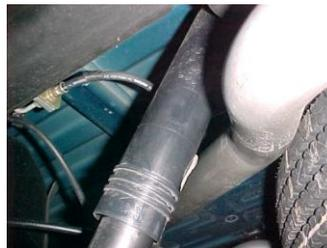
Install driverside overaxle tailpipe #E into muffler 1 1/2" to 2". Support end of tailpipe with jack stand and attach to hanger #H.
