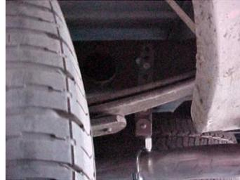
Install metal hangers # I into holes located approximately 22" from the rear of the frame. Metal hangers are mounted on the outside of the frame. Use bolt kit #K. The bolt and the washer will go into the 3<sup>rd</sup> hole from the top of the hanger.
