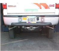
INSTALL PASSENGER SIDE TAILPIPE #C INTO MUFFLER AT LEAST 1 ½" TO 2". USE CLAMP #G TO SECURE PIPE TO MUFFLER. DO NOT TIGHTEN. THE TAILPIPES WILL BOTH LEAN TOWARDS THE DRIVER SIDE LOOKING FROM THE REAR OF THE VEHICLE - THIS TAILPIPE IS AT APPX. 11 O'CLOCK.
