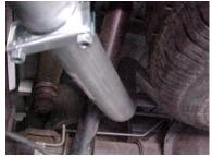
INSTALL DRIVER SIDE TAILPIPE #D INTO MUFFLER AT LEAST 1½" TO 2". THIS PIPE WILL ROUTE OVER THE AXLE AND BETWEEN THE SHOCK AND TIRE. ATTACH CLAMP #I TO SECURE TAILPIPE TO MUFFLER. DO NOT TIGHTEN. LOOKING FROM THE REAR OF THE VEHICLE - THIS TAILPIPE IS AT APPX. 11 O'CLOCK.
