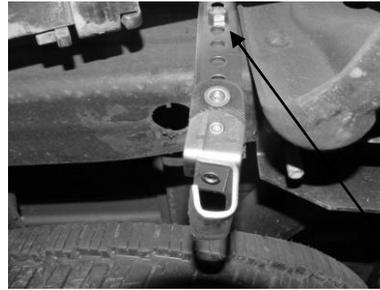
INSTALL METAL HANGERS #H INTO HOLES LOCATED APPROX. 16" FROM THE REAR OF THE FRAME. METAL HANGERS ARE MOUNTED ON THE OUTSIDE OF FRAME. USE THE HARDWARE PROVIDED. THE BOLT AND WASHER WILL GO INTO THE 3<sup>RD</sup> HOLE FROM THE TOP OF THE HANGER. YOU MAY NEED TO LOOSEN SPARE TIRE FOR EASIER REMOVAL.
