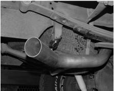
INSTALL TURNOUT PIPE # D ONTO OVERAXLE TAILPIPE USING CLAMP # E. INSERT WELDED HANGER INTO RUBBER GROMMET. DO NOT TIGHTEN.
