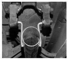
**UN-BOLT STOCK HEADPIPE** JUST BEHIND THE CATALYTIC CONVERTER. **DO NOT DAMAGE** STOCK BOLTS AND **GASKET! FOR YOU** WILL NEED TO RE-USE THEM. CUT OFF YOUR STOCK TAILPIPE JUST BEHIND THE MUFFLER AND REMOVE. LEAVE ALL RUBBER GROMMETS ON THE HANGER. USE WD-40 TO HELP WITH REMOVAL OF STOCK EXHAUST AND HANGERS.
