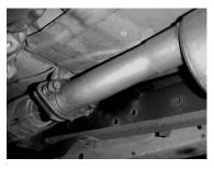
BOLT HEADPIPE #B TO THE FACTORY PIPE REUSING FACTORY BOLTS. DO NOT TIGHTEN. SLIP MUFFLER #C ONTO THE HEADPIPE NO MORE THEN 1" TO 2". THE INLET OF THE MUFFLER WILL BE LOOKING INTO THE LOUVERS. USE A JACKSTAND TO SUPPORT MUFFLER. ATTACH WITH CLAMP #G. DO NOT TIGHTEN.
