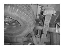
SLIP THE OVERAXLE TAILPIPE #E THROUGH THE LEAF SPRING IN BETWEEN THE SHOCK AND THE SWAY BAR. INSERT WELDED HANGER INTO RUBBER GROMMET.
