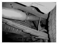
ROTATE OVERAXLE PIPE UNTIL YOU HAVE A MINIMUM OF A 1 " ON ALL PIPES FROM ALL RUBBER BRAKE LINES, TIRES, SWAY-BAR, SHOCKS, ETC. CLAMP DOWN WITH HANGER #D.
