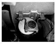
ONCE THE MUFFLER AND HEADPIPE ARE INSTALLED ROTATE THE MUFFLER AND HEADPIPE UNTIL MUFFLER OUTLET IS POSITIONED AT 4 O'CLOCK AND SITTING LEVEL UNDERNEATH THE VEHICLE. THEN TIGHTEN THE HEADPIPE. SLIP THE REAR WELDED HANGER INTO THE RUBBER GROMMET AND ATTACH TO MUFFLER USING HANGER #D.
