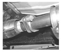
TO REMOVE EXHAUST- UN BOLT FLANGE LOCATED IN FRONT OF STOCK MUFFLER. DO NOT DAMAGE STOCK BOLTS, YOU WILL RE-USE THEM. NOW CUT OFF YOUR STOCK TAILPIPE JUST BEHIND THE MUFFLER AND REMOVE. LEAVE ALL RUBBER GROMMETS ON THE HANGER. USE WD-40 TO AID IN REMOVAL OF EXHAUST AND HANGERS.
