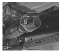
INSTALL FLANGE #G ONTO HEADPIPE #A. ATTACH TO FACTORY FLANGE RE-USING FACTORY BOLTS TO INSTALL IT. SNUG UP THESE BOLTS.
