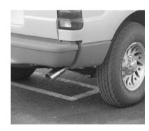
ROTATE TAILPIPE UNTIL YOU HAVE A MINIMUM OF 1 "FROM ALL PIPES, RUBBER BRAKE LINES, TIRES, SWAY BAR, SHOCKS, ETC. THEN TIGHTEN ALL CLAMPS AND HANGERS. REINSTALL THE REAR SHOCK MOUNT.
