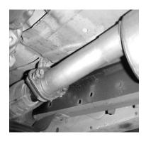
SLIDE FLANGE #D ONTO HEADPIPE #A AND BOLT TO FACTORY HEADPIPE REUSING FACTORY NUTS & BOLTS. (DO NOT TIGHTEN). OUTLET OF HEADPIPE SHOULD BE AT ABOUT 1'OCLOCK, SLIDE MUFFLER #B ONTO THE HEADPIPE NO MORE THEN 2" AND NO LESS THEN 1" ON THE INLET OF THE MUFFLER AND CLAMP WITH #G. MUFFLER INLET IS LOOKING INTO THE LOUVERS.
