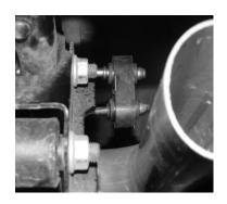
SLIP THE OVERAXLE PIPE #C THROUGH THE LEAF SPRING IN BETWEEN THE SHOCK AND THE SWAY-BAR AND INTO THE MUFFLER AT LEAST 1 ½" NO MORE THAN 2" USE HANGER #E TO CLAMP PIPE TO MUFFLER.
