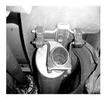
ONCE THE MUFFLER AND HEADPIPE ARE INSTALLED ROTATE THE MUFFLER AND HEADPIPE UNTIL MUFFLER OUTLET IS POSITIONED AT 3 O'CLOCK AND SITTING LEVEL UNDERNEATH THE VEHICLE. INSTALL THE O.E. HANGER #E ONTO OUTLET OF MUFFLER AND INSERT WELDED HANGERS INTO RUBBER GROMMET.
