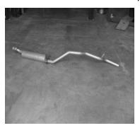
LAY OUT THE GIBSON EXHAUST AND COMPARE PART NUMBERS TO THE MANUAL. FOR AN EASIER REMOVAL LUBE ALL RUBBER GROMMETS WITH WD-40 AND CUT THE TAILPIPE DIRECTLY BEHIND THE MUFFLER. UN-BOLT THE FLANGE LOCATED IN FRONT OF STOCK MUFFLER. THEN REMOVE LEAVING ALL RUBBER GROMMETS IN PLACE, YOU WILL REUSE STOCK HEADPIPE FLANGE BOLTS.
