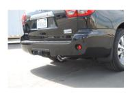
7. Install stainless steel tip. Clamp down. When you have everything in place, firmly tighten all bolts and clamps down securely. Use stainless steel cleaner and a Scotch Brite pad weekly to prevent tip from discoloration. Inspect all fasteners after 25-50 miles of operation and re-tighten as necessary. You may need to cut your stock tail pipe back to get your tip to fit correctly.
