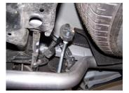
5. Install the over axle tailpipe #C into the muffler 1.5"-2". Use clamp #E to secure tailpipe to muffler. Do not tighten. Insert welded hangers into rubber grommets.
