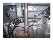
3. Install headpipe #A onto your existing stock front pipe and attach with clamp #E. Use a jack stand to support the converter. Insert welded hangers into rubber grommets.
