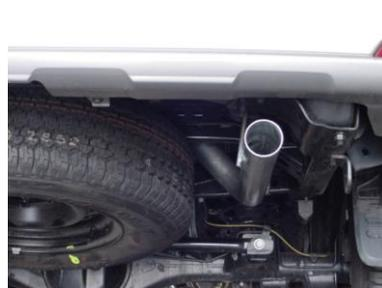
INSTALL EXITPIPE #D ONTO OVERAXLE TAILPIPE. INSERT WELDED HANGERS INTO RUBBER GROMMETS. USE CLAMP #H TO SECURE TO THE TAILPIPE. DO NOT TIGHTEN.
