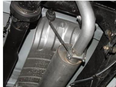
INSTALL HANGER #G INTO RUBBER GROMMET LOCATED JUST ABOVE THE OUTLET OF THE MUFFLER. USE THIS HANGER TO SECURE MUFFLER TO TAILPIPE. DO NOT TIGHTEN.
