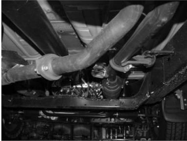
TO REMOVE STOCK EXHAUST UNBOLT THE CLAMP LOCATED BEHIND THE MUFFLER. THE TAILPIPE SHOULD SLIDE OFF. UNBOLT THE STOCK MUFFLER AND HEADPIPES FROM THE 2 FLANGES JUST BEFORE THE MUFFLER. DO NOT DISCARD STOCK NUTS AND BOLTS. LEAVE ALL RUBBER GROMMETS ON THE HANGER. USE WD-40 TO AID IN REMOVAL OF THE EXHAUST AND HANGERS.
