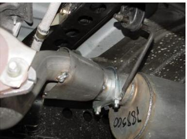
INSTALL FRONT MUFFLER HANGER #F INTO RUBBER GROMMETS LOCATED JUST ABOVE THE INLET OF THE MUFFLER. USE THIS CLAMP TO SECURE HEADPIPE. DO NOT TIGHTEN.
