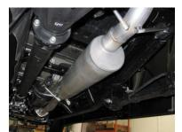
**INSTALL MUFFLER #B** ONTO HEAD PIPE 1-1/2" TO 2" WITH THE LOUVERS FACING TOWARDS THE CONVERTER. THE MUFFLER OUTLET SHOULD **BE POSISTIONEDTHE** MUFFLER OUTLET SHOULD BE POSITIONED AT 12:00. USE A JACK STAND TO SUPPORT THE MUFFLER. **USE CLAMP #E TO SECURE** THE MUFFLER TO THE HEAD PIPE. DO NOT TIGHTEN. MUFFLER INLET IS LOOKING INTO THE LOUVERS.
