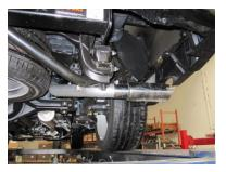
NEXT INSTALL REAR MUFFLER HANGER #G ONTO OUTLET OF MUFFLER. INSERT WELDED HANGER INTO RUBBER GROMMETS
