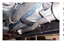
LAY OUT THE EXHAUST ON THE FLOOR SO IT LOOKS LIKE THE DRAWING AND COMPARE PARTS WITH MANUAL. TO REMOVE THE STOCK EXHAUST REMOVE IT FROM THE 2-BOLT FLANGE LOCATED IN THE FRONT OF THE MUFFLER. LEAVE ALL RUBBER GROMMETS IN PLACE. USE WD-40 TO AID IN REMOVAL OF EXHAUST AND HANGERS.
