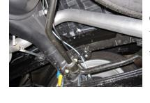
INSTALL THE OVERAXELE TAILPIPE #C INTO THE MUFFLER 1-1/2" TO 2". DO NOT TIGHTEN.
