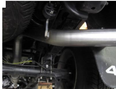
ALUMINUM OR STAINLESS STEEL CLEANER TO POLISH YOUR TIP. MAKE SURE YOU HAVE A MINIMUM OF A 1" CLEARANCE ON ALL PIPES FROM ALL RUBBER BRAKE LINES, TIRES, SHOCKS, FUEL LINES, ETC. THEN TIGHTEN ALL CLAMPS AND HANGERS
