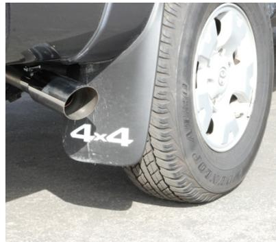
**"MAKE SURE YOU HAVE A MINIMUM OF A 1" CLEARANCE ON ALL PIPES FROM ALL RUBBER BRAKE LINES, TIRES, SHOCKS, SPARE TIRE, FUEL LINES, ETC."**
