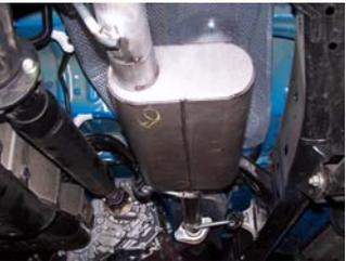
3. Install muffler #B onto head pipe 1½"-2" with the louvers facing towards the converter. Use a jack stand to support the muffler. Use clamp #F to secure the muffler to the headpipe. DO NOT TIGHTEN.
