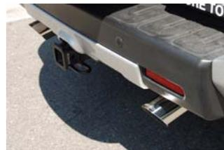
7. Install stainless steel tip #E. Clamp down. When you have everything in place, firmly tighten all bolts and clamps down securely. Use stainless steel cleaner weekly to prevent tip from discoloration.
