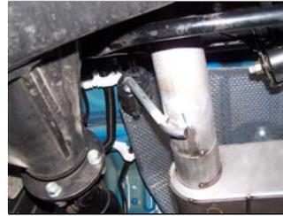
4. Install the overaxle tailpipe #C into the muffler 1½-2" secure with clamp #F. DO NOT TIGHTEN. Insert welded hanger into rubber grommet.
