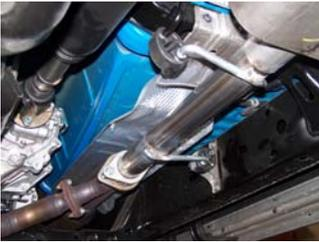
2. Install head pipe #A onto your existing stock front pipe and attach with hardware kit #G. DO NOT TIGHTEN. Insert welded hangers into rubber grommets.
