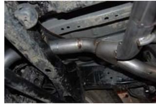
5. Next, install the Y-Pipe #D. onto overaxle pipe. Use clamp #F to secure to the tailpipes. DO NOT TIGHTEN. Insert welded hanger into rubber grommet.
