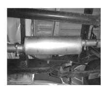
SLIP MUFFLER #B ONTO HEADPIPE NO MORE THEN 2" AND NO LESS THEN 1". ATTACH TO HEADPIPE WITH CLAMP #F. THE MUFFLER INLET WILL HAVE THE INSIDE LOUVERS FACING FORWARD. THE OUTLET OF THE MUFFLER WILL BE POSITIONED AT 12 O'CLOCK. USE A JACK STAND TO SUPPORT THE MUFFLER. THE MUFFLER INLET IS LOOKING INTO THE LOUVERS.
