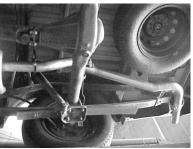
SLIP THE OVER AXLE TAILPIPE #C INTO THE OUTLET OF THE MUFFLER NO MORE THEN 2" AND NO LESS THEN 1". INSERT WELDED HANGER INTO RUBBER GROMMET.
