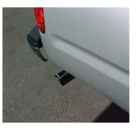
NEXT INSTALL YOUR STAINLESS STEEL TIP TO YOUR DESIRED LOOK. USE ANY ALUMINMUM OR STAINLESS STEEL CLEANER TO POLISH YOUR TIP. MAKE SURE YOU HAVE A MINIMUM OF A 1" CLEARANCE ON ALL PIPES FROM ALL RUBBER BRAKE LINES, TIRES, SHOCKS, FUEL LINES, ETC. THEN TIGHTEN ALL CLAMPS AND HANGERS
