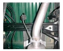
INSTALL REAR MUFFLER HANGER #E INTO THE RUBBER GROMMETS LOCATED ABOVE THE MUFFLER OUTLET. THE VERTICAL RODS WILL BE FACING TOWARDS THE REAR OF THE TRUCK. DO NOT TIGHTEN. THIS CLAMP WILL BE USED TO SECURE TAILPIPE TO MUFFLER
