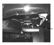
INSERT HANGER INTO RUBBER GROMMET.
