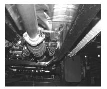
BOLT HEADPIPE #A TO STOCK FLANGE. RE-INSTALL O2 SENSOR USING FACTORY GASKET, INTO HEADPIPE BEHIND FLANGE AND USE BOLT KIT #G TO ATTACH. WE RECOMMEND TO USE O2 SENSOR SAFE GASKET SEALER TO HELP PREVENT LEAKS.
