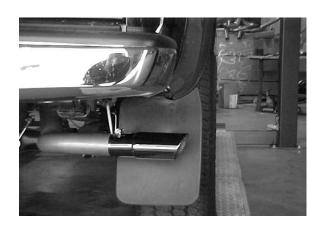
INSTALL THE STAINLESS TIP. USE A STAINLESS OR ALUMINUM CLEANER TO POLISH TIP. NOW TIGHTEN ALL HANGERS AND CLAMPS.
