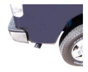
8. Install stainless steel tip. Clamp down. When you have everything in place, firmly tighten all bolts and clamps down securely. Use stainless steel cleaner and a Scotch Brite pad weekly to prevent tip from discoloration. Inspect all fasteners after 25-50 miles of operation and re-tighten as necessary. You may need to cut your stock tail pipe back to get your tip to fit correctly.
