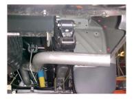
INSTALL EXIT PIPE #D ONTO TAILPIPE. MAKE SURE ITS LEVVEL. USE CLAMP #G TO SECURE PIPES TOGETHER. DO NOT TIGHTEN.
