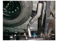
SLIP OVERAXLE PIPE #C INTO THE OUTLET OF THE MUFFLER NO MORE THEN 2" AND NO LESS THEN  $1\frac{1}{2}$ ". THE SPARE TIRE MAY NEED TO BE LOSENED AND PUSHED TO THE REAR OF THE TRUCK TO GAIN CLEARANCE FOR INSTALLATION OF OVERAXLE PIPE. INSERT WELDED HANGER INTO RUBBER GROMMET.
